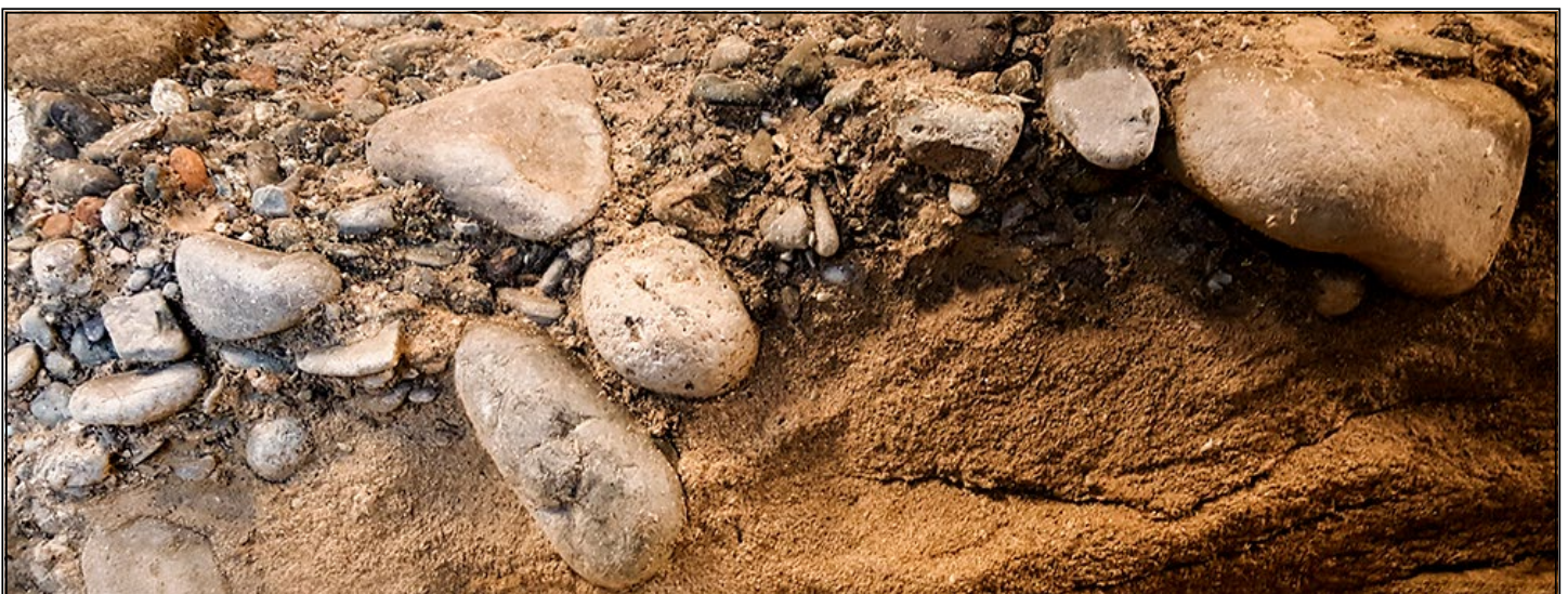
Cross section of large chunk of embedded gravel. Note the layers of small gravel (top), a layer of gravel, and a thick layer of sand and fines. Collected from a section of Lower Putah Creek in an area that is plagued by embedded and cemented gravel.
