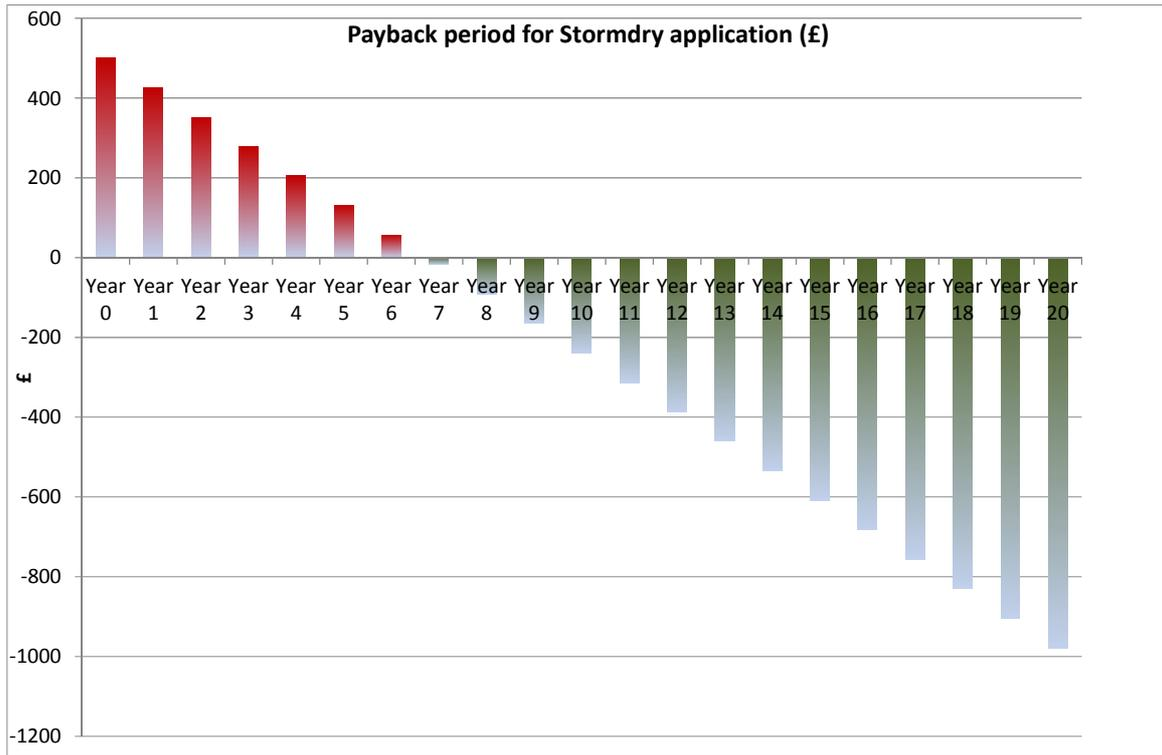
Figure 4. Payback period for Stormdry treatment including materials and labour
