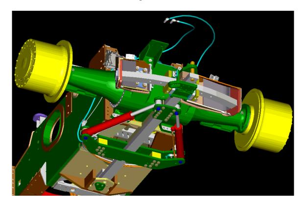
The **Damped mode** is accomplished by placing the tractor SCV in the "Float" position. (See tractor Owners Manual for Tractor Control information) The Drawbar will now be allowed to float from side to side at a controlled rate within the limits of the tractor drawbar locking clamps provided with the tractor. Variable damping rates are available if other than what is provided is desired. (Contact AJ Equipment for parts and installation information.)
