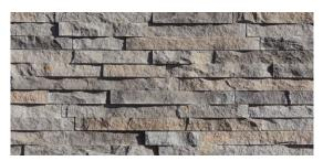
European Ledge consists of 1.5" precision-cut ledge stones molded into 4.5"H × 24"W panels. A stair-stepped edge creates a tight-fit, eliminating unsightly vertical joints.
