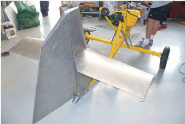
The tails are all aluminum and come Ready built and primed or painted
