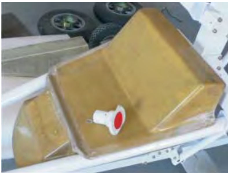
The ARAMID (Kevlar) reinforced fuel tank was tested to withstand 15G and is protected by the triangulation of the frame.
