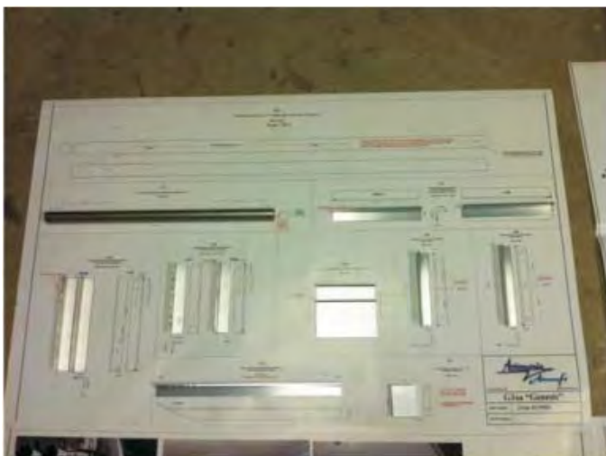
Assembly booklet and drawings are supplied with the kits as well as videos with step by step demonstration of the complete assembly.
