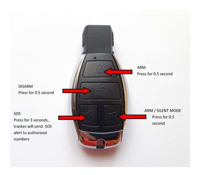
Press the ARM button on the remote control for 0.5 second, the vehicle enters into armed state and the siren will beep once. If the ignition is switched on (ACC on) then the vehicle will not ARM.
