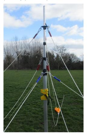
Attach the wind sensor and lay any sensor connecting cables towards the wind speed / direction display.
