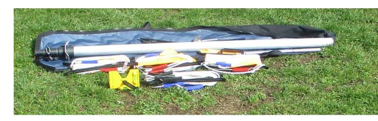
The mast equipment is presented in a zippered valise with a carry handle for ease of storage and transportation, containing the mast base spigot rod, claw hammer, all guy lines, ground pegs and a vertical spirit level.
