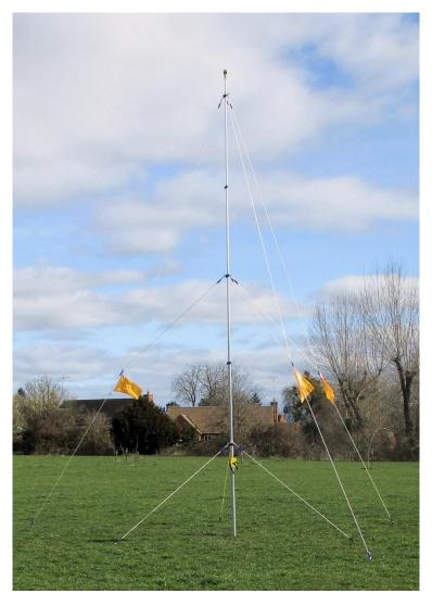
The 7m telescopic mast system has been tested with our full range of wind sensors in wind speeds of 25m/s, 90Kmh, 55.9Mph with no sensor deviation.
