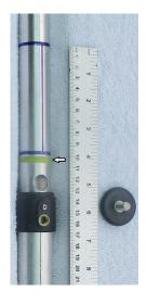
The mast has round screw threads that screw through the mast into a locking hole, these holes stop the mast from being over extended.
