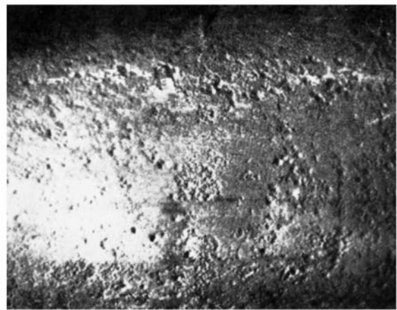
Figure 10 - General Corrosion with Pitting on Cylinder Wall
