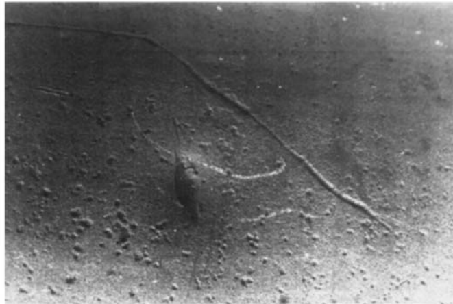
Figure 5 - Dent with Isolated Pitting
