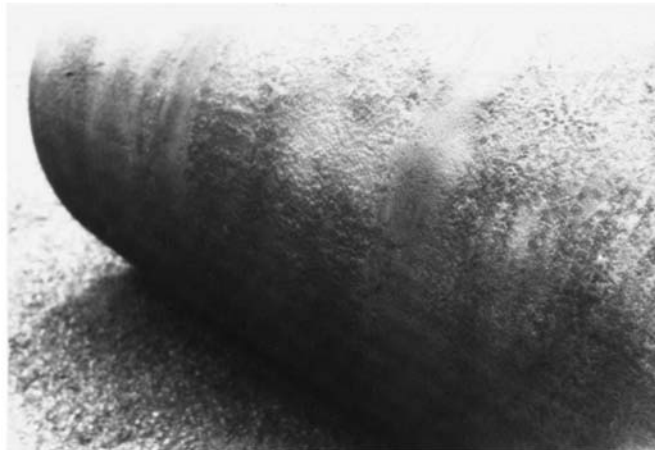
Figure 7 - Line Corrosion - Cylinder Wall
