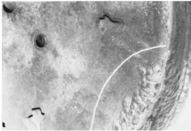
Figure 11 - Chime Corrosion Ton Container Head
