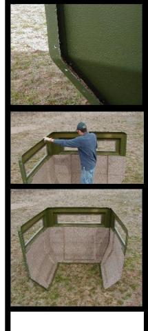
6. Then attach the door panel and secure it the same way. At this point you should have the three window wall panels and the door panel standing and loosely attached to each other.
