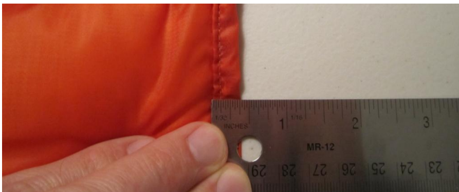
Hemming side seam, \frac{3}{8} " wide sewn \frac{1}{4} " from edge.
