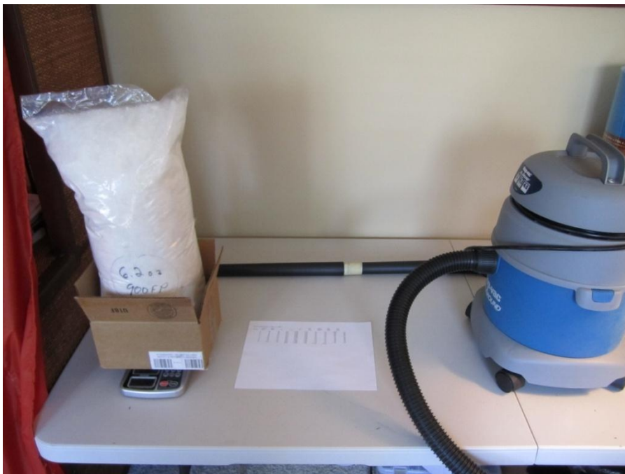
Down filling station: shop vac, scale, printout, down (in box). Note that no-seeum netting is taped over next to last extension
