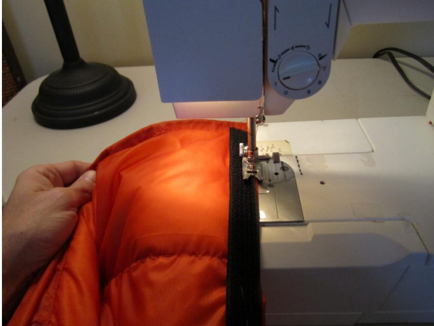
Sewing the Velcro in place.
