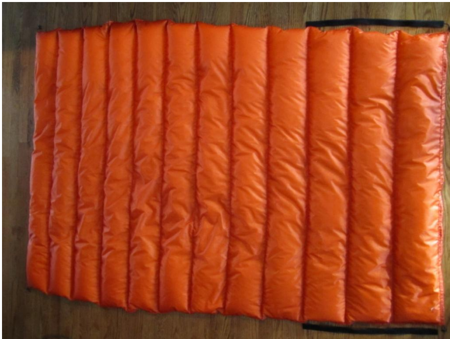
Quilt with chamber full, edges hemmed, with Velcro place next to location for sewing.
