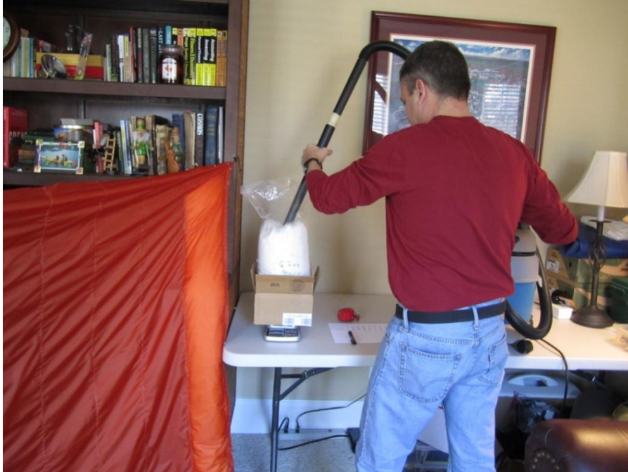
Vacuuming the down into the extension. Down is stopped by the no-seeum netting
