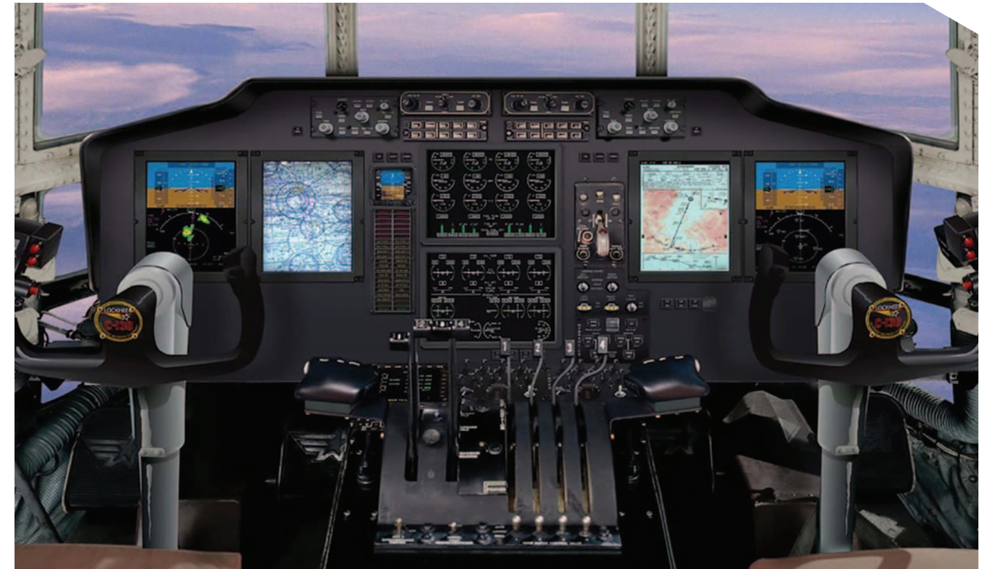
▲ Shown here is the cockpit of a Portuguese Air Force C-130H recently upgraded by Collins Aerospace of Cedar Rapids, Iowa, with the Flight 2 avionics upgrade. (Image courtesy of Rockwell Collins.)
