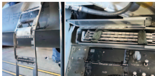
A group of airmen at Aviano Air Base in Italy are pitching an idea for a folding boarding ladder that F-16 pilots can stow in the map case in the jet's cockpit. (photo courtesy U.S. Air Force)
