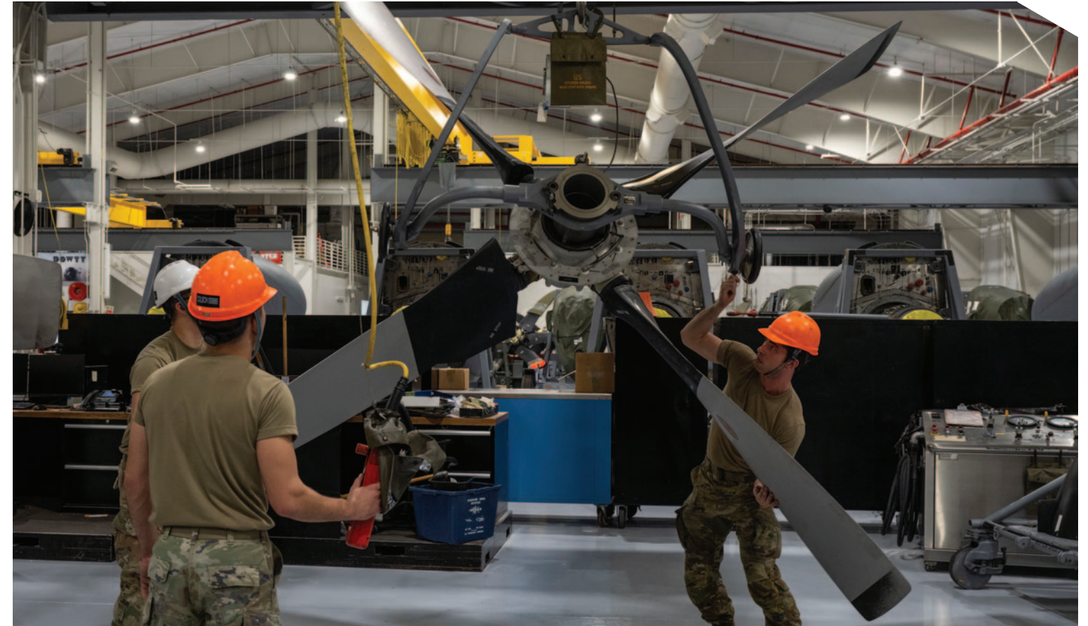
▲ U.S. Air Force technicians work on the rear spinner of a MC-130 H. While ex-military technicians make highly desirable employees for aftermarket MRO firms, their numbers are not equal to the industry’s current need for workers. (Photo by Airman 1st Class Hussein Enaya, U.S. Air Force.)
