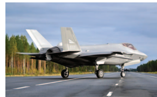
A Norwegian F-35A fighter jet takes off after a touch-and-go landing on a highway in the Finnish forests. Immediately after landing, so-called "hot pit refueling" was carried out – a technique in which the motor runs while the fuel tank is being filled in order to reduce downtime. (Photo: Ole Andreas Vekve/the Norwegian Armed Forces)
