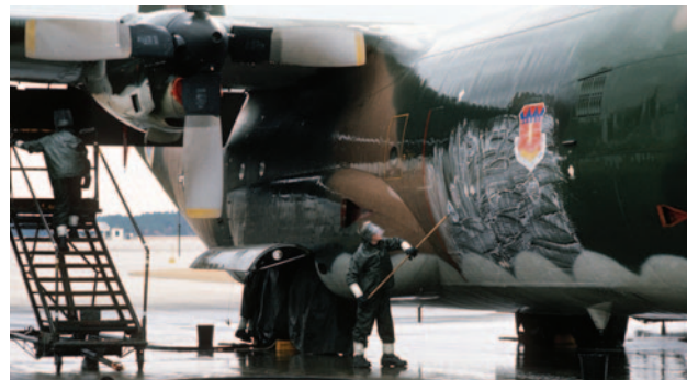
A C-130 maintainer washes the fuselage of a C-130 Hercules — in just one of many regularly scheduled maintenance tasks. (National Archives and Records Administration.)
