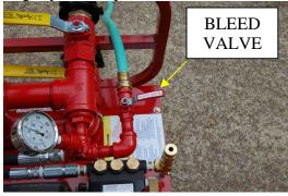
Now open the inlet (hydrant) valve. Do not increase the pressure at the pump panel if using a pumper truck. Truck can remain at idle, it is only filling the hose.
