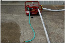
Hose being tested should have either a nozzle or a drain cap attached. Make sure motor is off at this time.
