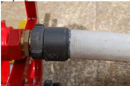
Attach hoses to test machine. You can put as much as 150' per each connection. Make sure you have a large enough fairly clean area to do this. Do not use another extension cord other than the one provided or do not add to it. Stretch out drain green drain hose or you will get wet.
