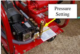
Once the pressure is reached, open the valve for the test hose, allow to reach test pressure and then close valve. Do this one at a time for each section attached. Once pressure has been reached close all ball valves and shut pump **OFF.**
