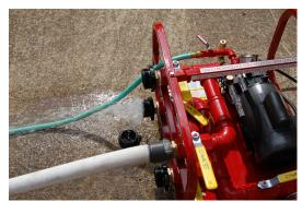
With the bleed valve open, turn on the pump at the switch
