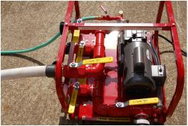
Open nozzle or drain cap and bleed all air out of the line.
