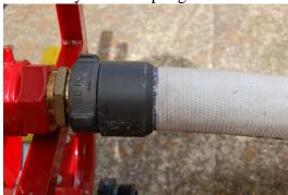
After test time, slowly open nozzle or test cap to relieve pressure then crack open bleed valve. Mark any failed hoses and take them out of service. Record hoses successfully tested per you department SOG's.
