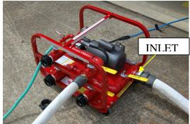
Mark around each coupling with a sharpie marker. This will be used later to make sure hose is not slipping in
