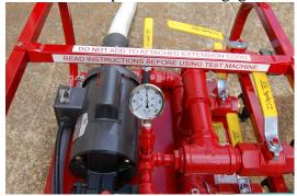
If necessary to change the pressure, you can adjust the pressure valve by backing off the jamb nut and rotating the valve, make sure the jamb nut is tightened back. This adjustment must be made when there is no pressure in the system. If you need to change pressure setting, bleed all test hoses and the bleed valve and then adjust.
