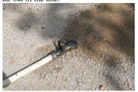
Once **ALL** air is out of line, first close the nozzle at one end of the hose and then the valve at the tester. Repeat this for each section being tested. Even if a connection is not being used, crack the valve open to drain any air in the system. See picture on next page.
