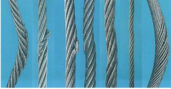
Loose, kinked, crushed, bird caged wire rope, waviness (more than 4/3d) or any damage resulting in distortion of the rope structure.
