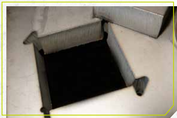
60 mm cut with WMS (using N 2 plasma and water secondary) at 800 A
