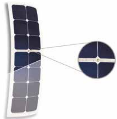
Custom panel with laminated bypass diodes, to minimize shading effects on a flexible panel without junction box
