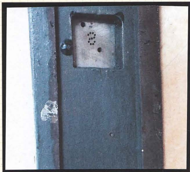
Scan of the underside of the base plate drilled to accept the hollow pins arranged like an "S". The small circles of paper cut by the hollow pins would eventually fall out of the perforating machine.
