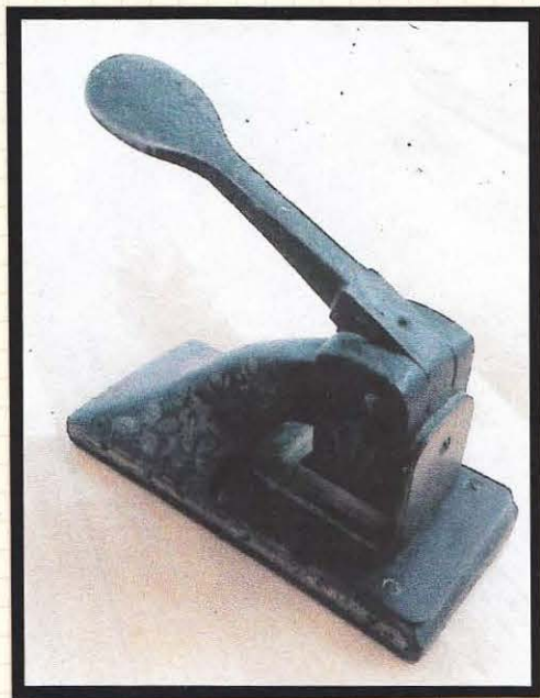
Scan of the machine used to perforate stamps one by one
