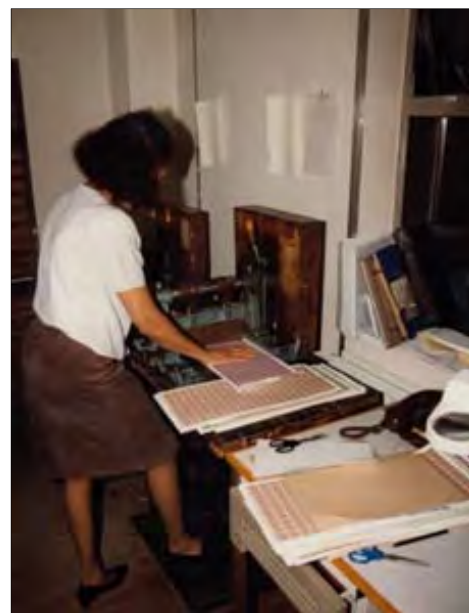
Using the treadle indexing mechanism to forward the sheet to the next stroke of the die head
