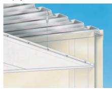
Cutaway section of corrugated roof deck and acoustical ceiling.
