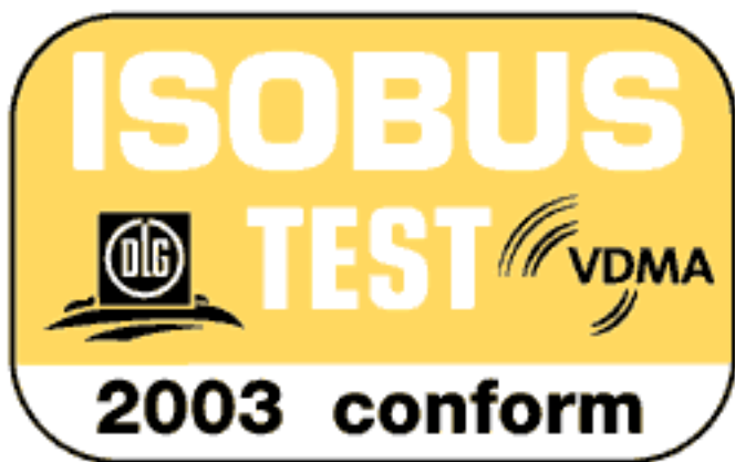
Figure 4.2.1b2. Electrical components that are ISO 11783-ready will be indicated by an ISOBus approval label (source: ISOBus website www.isobus.net ).
