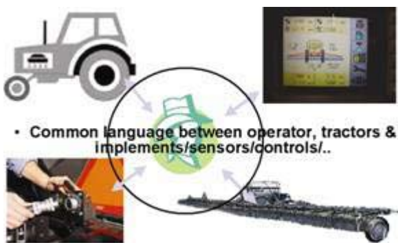
Figure 4.2.1b1. Examples of the types of equipment that need to be linked electronically. (source: Rudi Bartels BeeLine Technologies).
