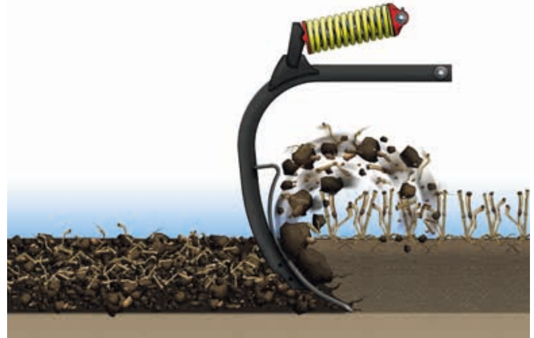
With the MixIn shin, the material in the entire cultivated horizon is crumbled finely and mixed.
