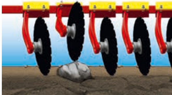
The discs are individually fitted to maintenance-free rubber suspension. This improves precision in the vertical and horizontal directions and gives good throughflow.
