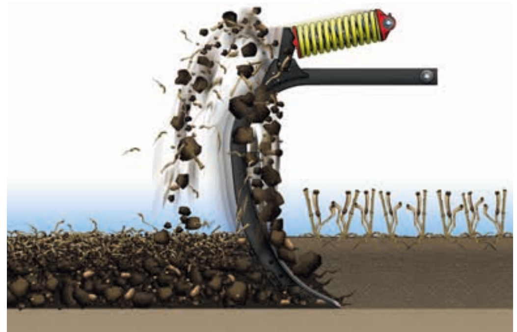
The Twist shin leaves a larger proportion of crop residue in the surface layer.
