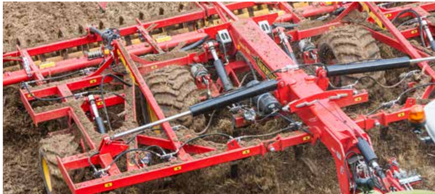
When equipped with DeepLoosening points, Opus can break pans down to a depth of 40 cm. To decrease the draught requirement, Opus can also be fitted with LowDisturbance points and folding tines.
