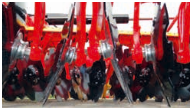
The discs are individually fitted to maintenance-free rubber suspension. This improves precision in the vertical and horizontal directions and gives good throughflow.
