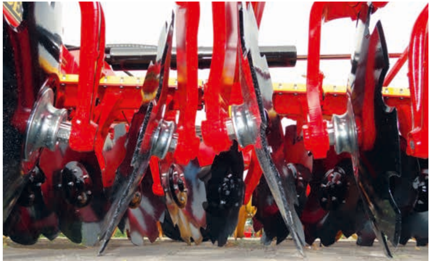
The X-shape gives the machine a soil-seeking mode of operation and keeps it running in an impressively straight line.
