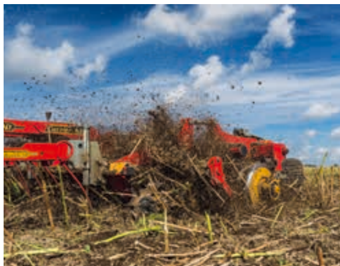
CrossCutter Disc works best at high speed.
