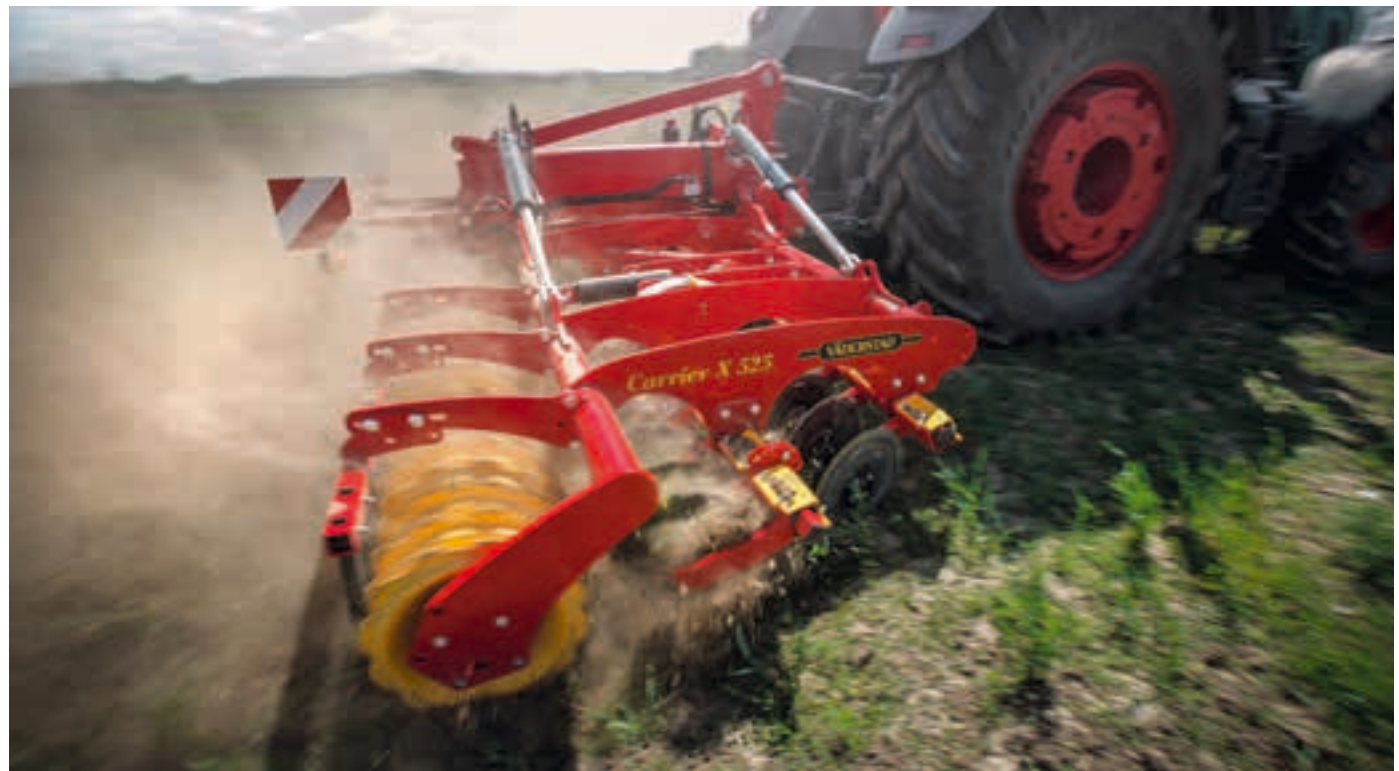
The positioning of the discs in an X-shape ensures stability and permits operation with GPS. The disc angle ensures good penetration capacity.
