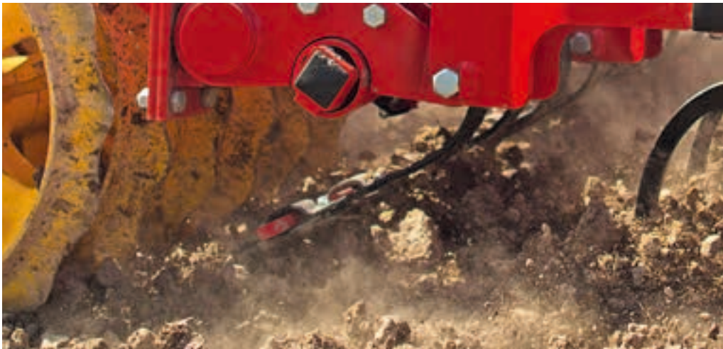
CrossBoard with double-acting stabiliser bar is used in ploughed cultivation to crush clods and level the surface. If CrossBoard is used during stubble cultivation for levelling purposes, this should take place without the stabiliser bar.
