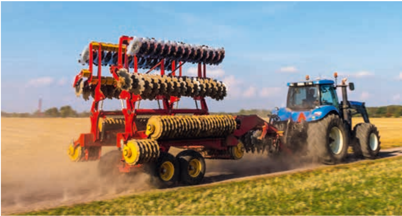
Carrier L and XL 9.25 and 12.25 have Väderstad folding. All models have a transport width of only 3 m.
