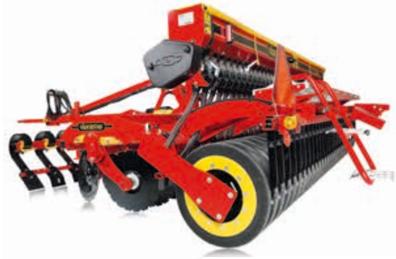
BioDrill BDX 180 or 250 is a flexible mechanical seed hopper and has a studded feed system that permits the seed to fall under its own weight.
