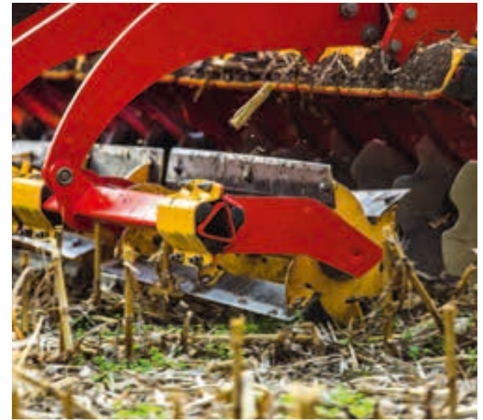
Short knife blades and small base roller diameter guarantee good responsiveness and high rotation speed during the work.
