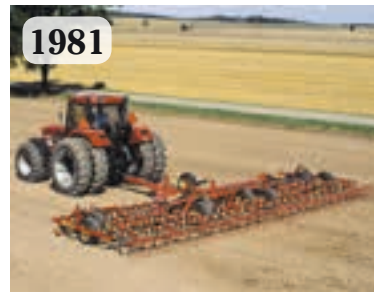
The NZ harrow is probably the most successful series of harrows ever made. It is characterised by high capacity, great durability and fewer passes being required than previously.
