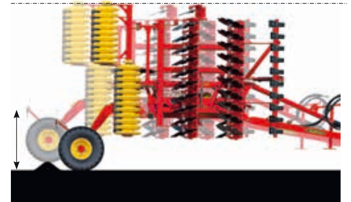
Transport suspension for the wheels, where the transport wheel cylinder is connected to an accumulator that ensures the machine runs smoothly, is standard for Carrier L and Carrier XL 425-825.
