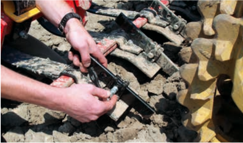
SingleKnife knife tool. Fitting to the CrossBoard points is simple when you use the Väderstad QuickChange System.
