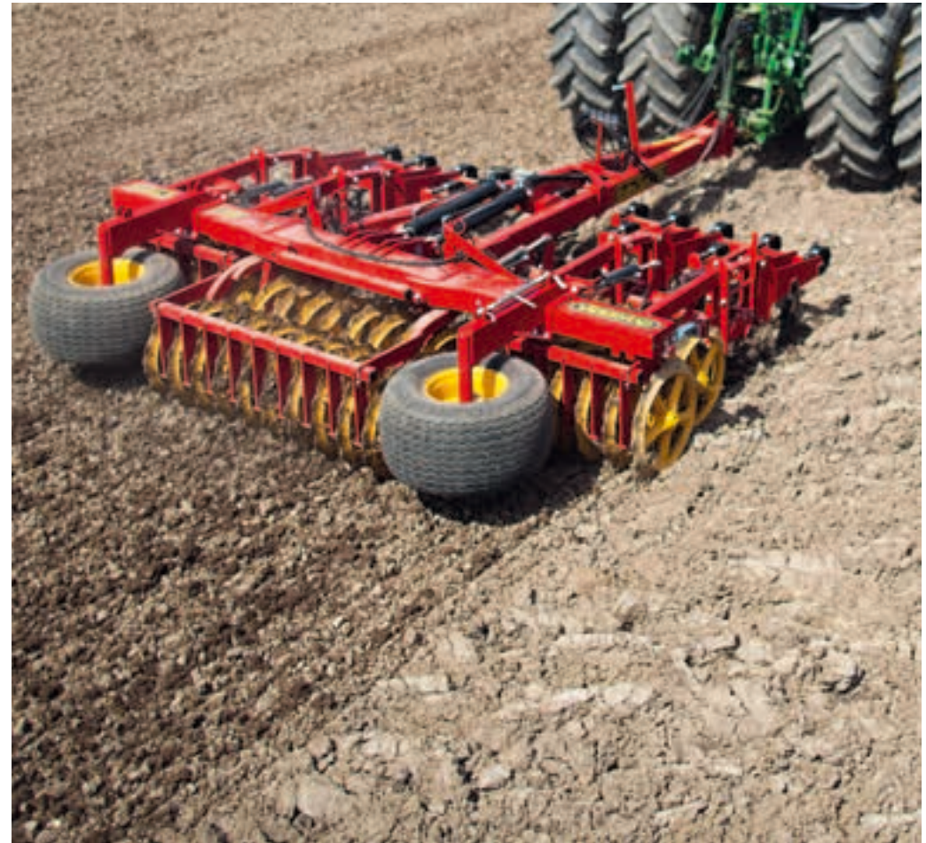
To increase the tine spacing in the front tool, the packer can be upgraded by adding a third axle. This gives better soil flow and more throughflow of straw and crop residue.
