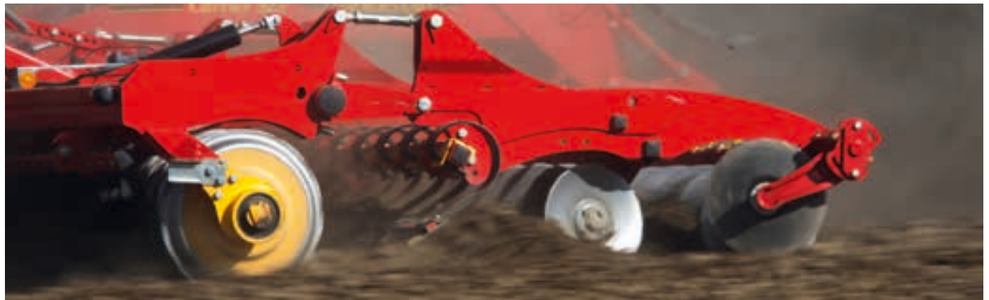
CrossBoard's double-acting stabiliser bar enables levelling in two directions, forwards and backwards.
