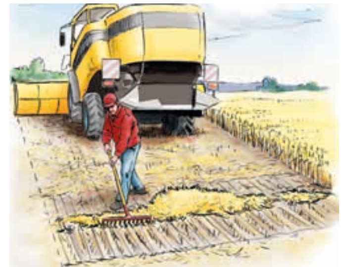
Do you have good straw distribution after harvesting? Test this by raking up a 1 m strip across the entire width of the harvester.
