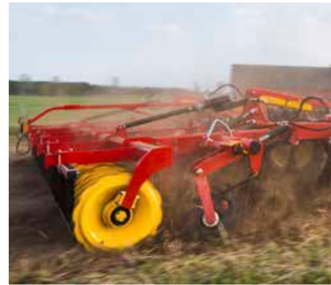
SteelRunner breaks surface straw and presses it into a shallow surface layer in order to achieve optimal decomposition rate.
