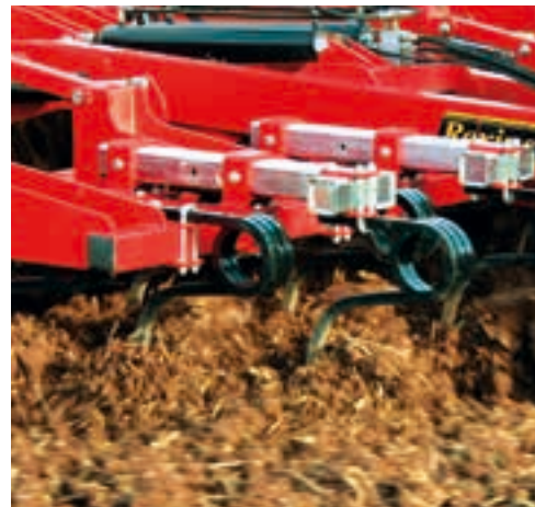
To increase the tine spacing in the front tool, the packer can be upgraded by adding a third axle. This gives better soil flow and more throughflow of straw and crop residue.
