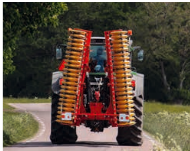
Folded in the transport position, Carrier X is only 2.4 m wide and has impressive ground clearance.
