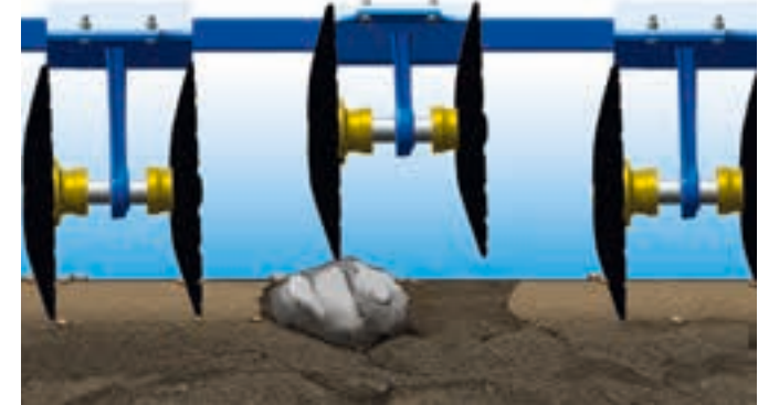
Having two discs per arm decreases throughflow and compromises precision.
