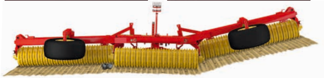
The roller sections are freely jointed from each other, which allows large obstacles to be overcome in the field without affecting the responsiveness. The design solution with a more robust frame compared with centre-suspended rollers gives a more uniform work result, and stones are pressed down more efficiently.
