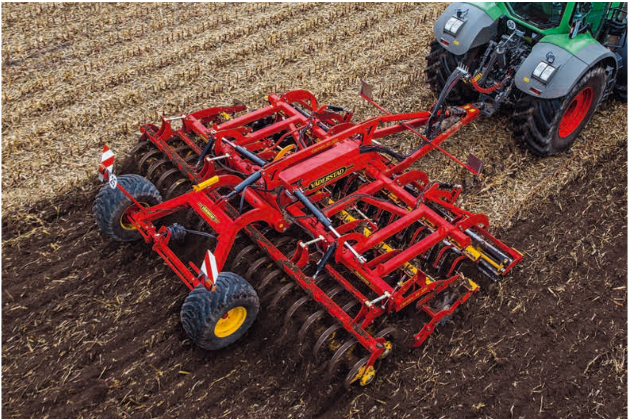
The robust frame and 61 cm discs give Carrier XL the weight and power required in fields with dense crop residue.
