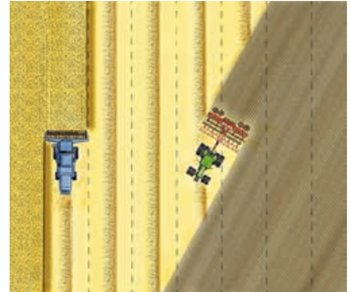
Carrier with a straw harrow is driven diagonally to the harvesting direction.
