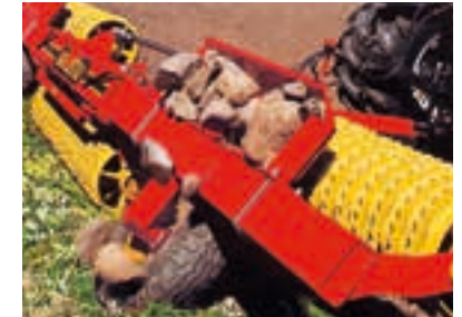
They are easy to empty from the cab using the roller's hydraulics.
