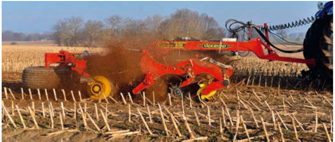
CrossCutter Knife and CrossCutter Disc in combination combats corn borers effectively by cracking corn stalks. The SteelRunner that follows crushes the residue and mixes it with the soil.
