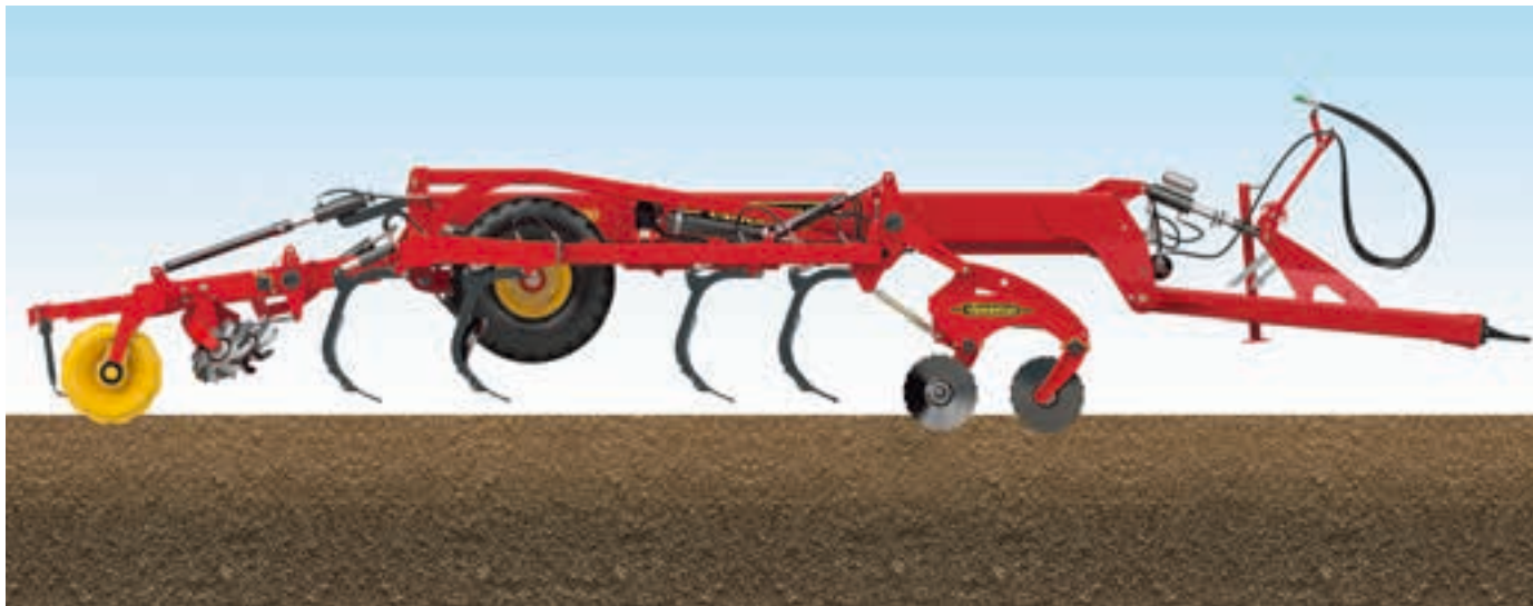
Shallow cultivation, only discs and packer working.
