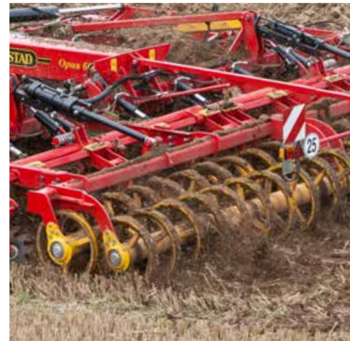
Double SoilRunner is a U-profile packer where soil works against soil.
