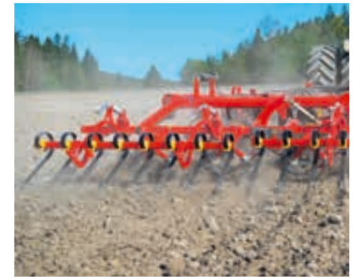
Swift can be equipped with either 12 mm following harrow tines or powerful, spring-suspended tiller tines of 9.5 x 45 mm. It is possible to switch between the two trailing implements.
