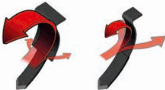
Shin width determines the amount of soil mixed.
