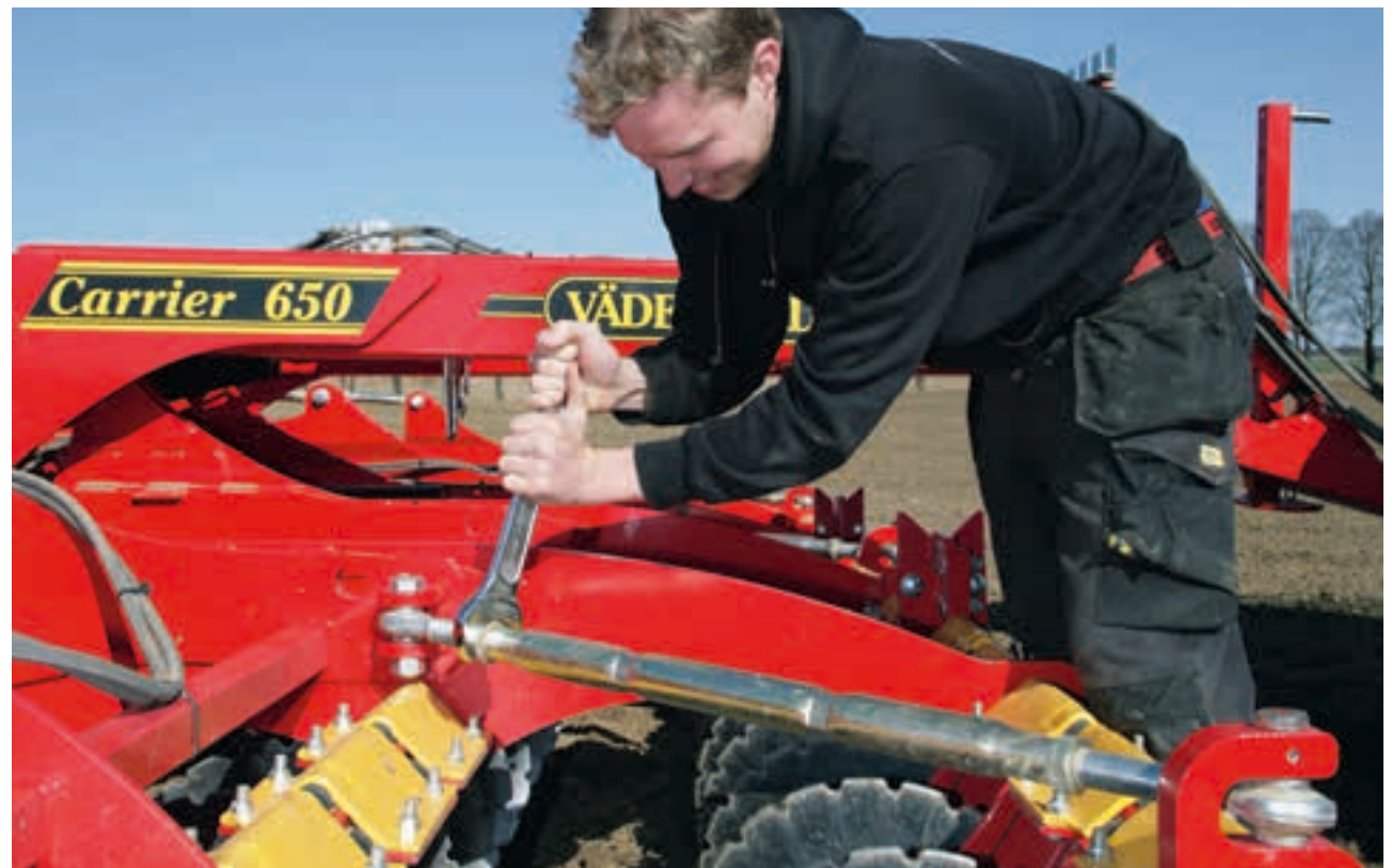
The axles are adjustable in the lateral direction for optimal work results.
