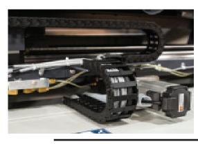
Pneumatic lines and electrical wiring are encased in industrial cable track.
