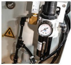
Regulator, filter and primary shut off value for easy pneumatic connection.
