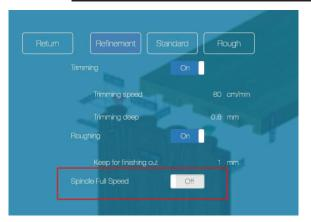
Programs allow for profile specific RPM and feed systems.
