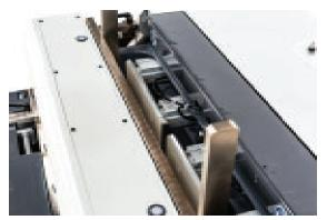
• Both vertical part clamps are bi-directionally powered for quicker part change.
