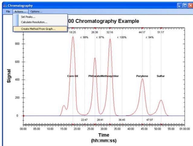
Annotate the chromatogram, dragging the resolution lines to the desired cut points as described above for the desired analytes. From the chromatography window, select “Actions”, then “Create Method from Graph”.
