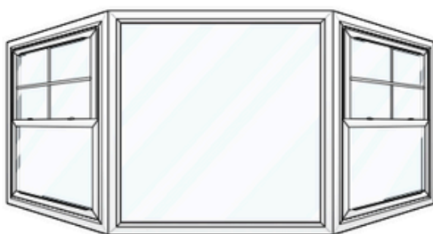
Bay: 3-Lite Unit with 2 Operable Windows with Screens
