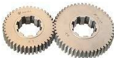
Pairs of feed and speed gears
