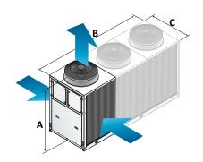
EVV - Outdoor unit with single heat exchanger and vertical airflow
