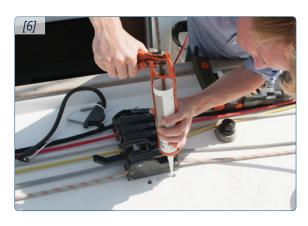
Place the Constrictor® base on the holes, avoiding contact between the textile sleeve and fresh sealant.
