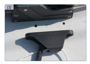
Drill the marked holes with 8mm (5/16") drill bit for CT306/CT308/CT310 models or, the 12mm (1/2") drill bit for CT312/CT314 models.
