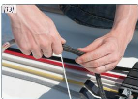
1 4 Hook the elastic loop to the end of the textile sleeve. This pre-tension on the sleeve helps to ensure a positive initial grip when transferring the load on the line or halyard from the winch to the Constrictor®. Manually "milking" the textile sleeve in the direction of the load prior to releasing from the winch will minimise movement of the line as the load is taken up by the Constrictor®.
