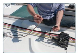
13 Thread the rope through the entire length of the textile sleeve until it comes out the other end of the body.
