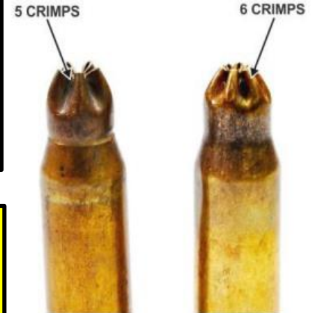
Figure 87. Grenade Cartridge vs. Blank Cartridge
