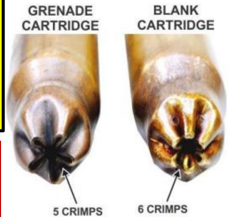
Figure 88. Grenade Cartridge vs. Blank Cartridge
