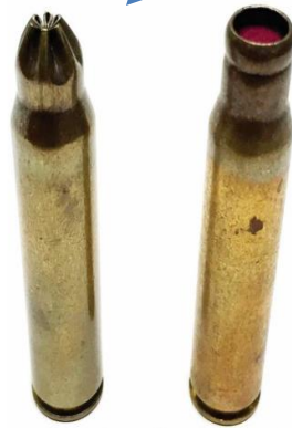
Figure 86. Authorized ammunition – rosette crimp (left) bottle nose (right)
