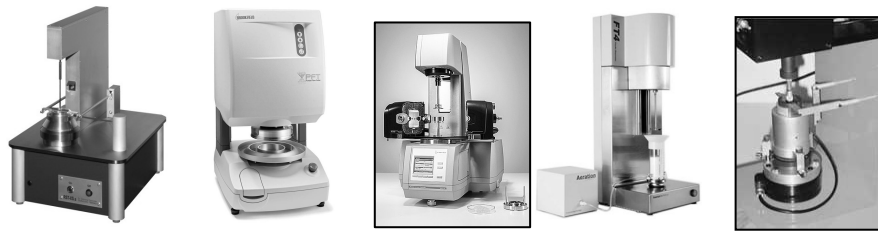
Figure 4.4. Automated testers; left to right: Schulze, Brookfield Engineering and Anton-Paar annular ring shear testers, Freeman Technology and E&G Associates (Peschl) torsional testers.
