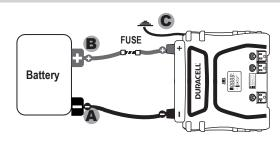
Fuse size 2000 Watt Inverter: ANL-200 3000 Watt Inverter: ANL-300
