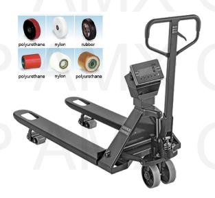
Hydraulic pumps on these trucks help you easily raise and move pallets. The forks are rounded and have a cutout for the load wheels. The handle has a three-position hand control (raise, lower, and neutral). A relief valve prevents pressure build-up to provide overload protection.
