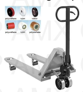
Hydraulic pumps on these trucks help you easily raise and move pallets. The forks are rounded and have a cutout for the load wheels. The handle has a three-position hand control (raise, lower, and neutral). A relief valve prevents pressure build-up to provide overload protection.
