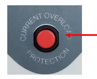
Example Overload Switches (Press to Reset)
