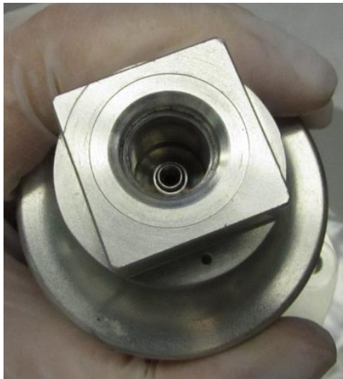
Flow Control in Actuator Port
