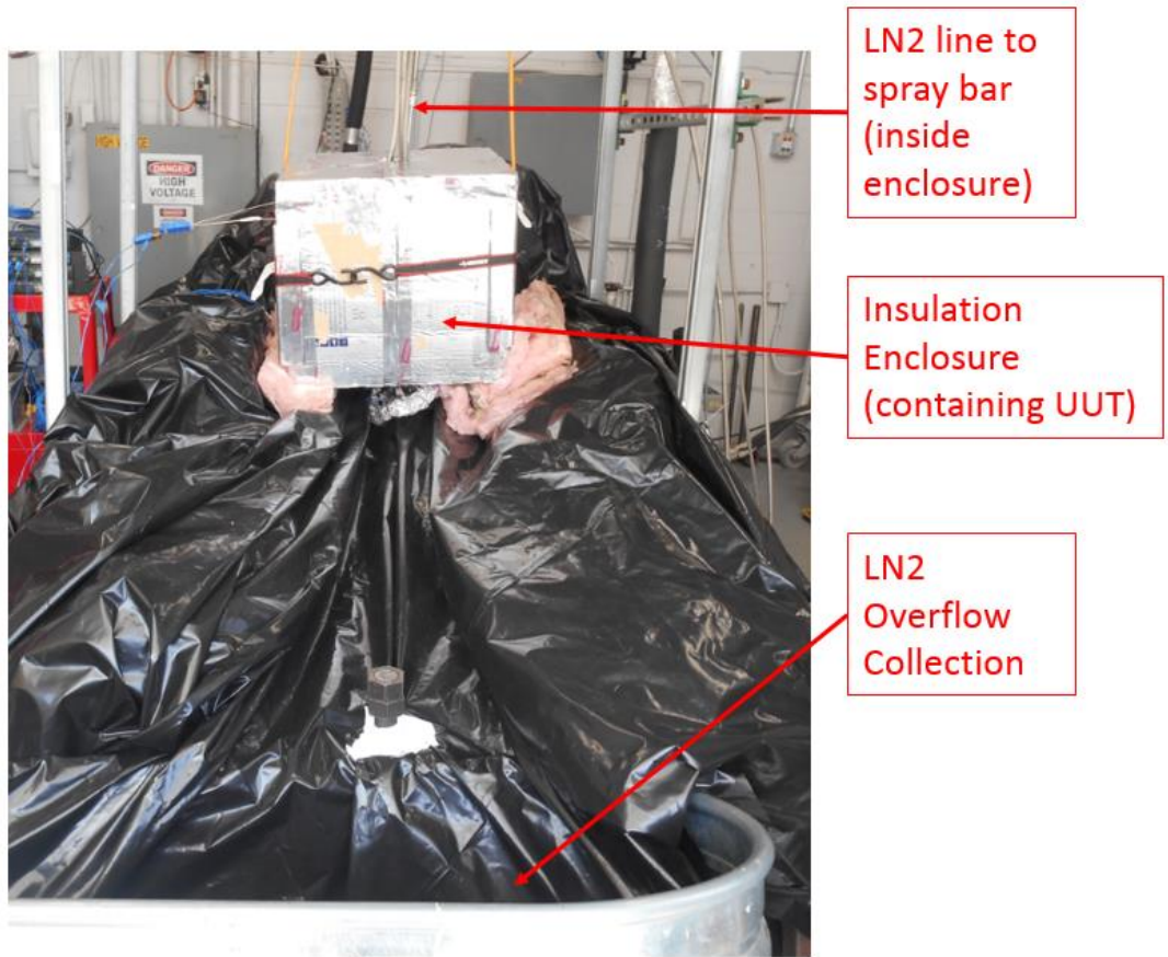
FIGURE 21 X-AXIS VIBRATION TEST CRYO SETUP
