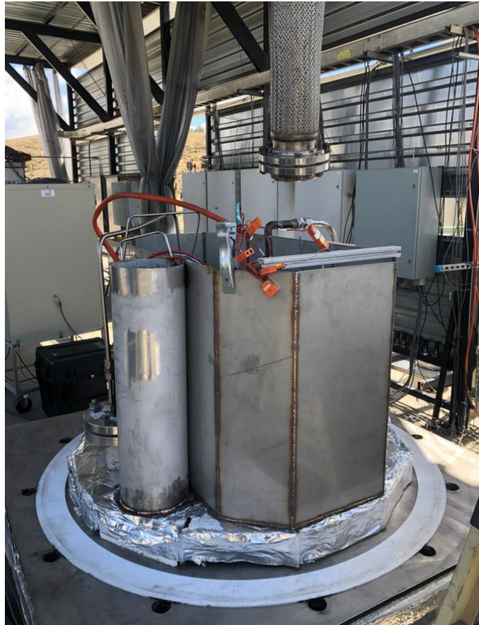
FIGURE 47 POST-OP LIFE TESTS: TEST SETUP (PRIOR TO CLOSING BELL JAR)
