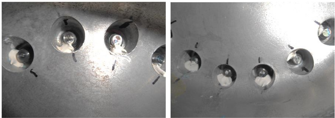
FIGURE 22 X-AXIS VIBRATION: PRE-TEST TORQUE STRIPE
