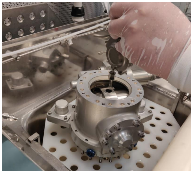
FIGURE 58 PARTICLE GENERATION TEST: IPA FILL AT INLET
