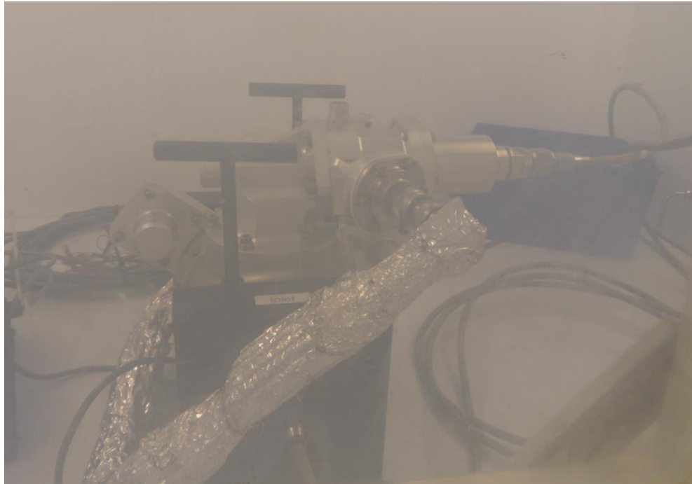
FIGURE 65 BURST PRESSURE TEST: ACTUATOR
