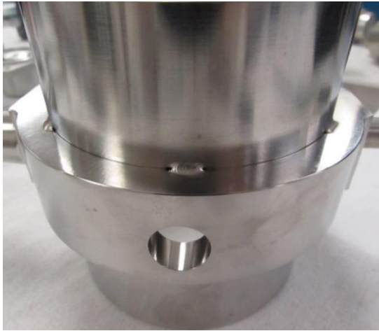
FIGURE 126 FLOW GUIDE WELDMENT: WELDED LOCATIONS
