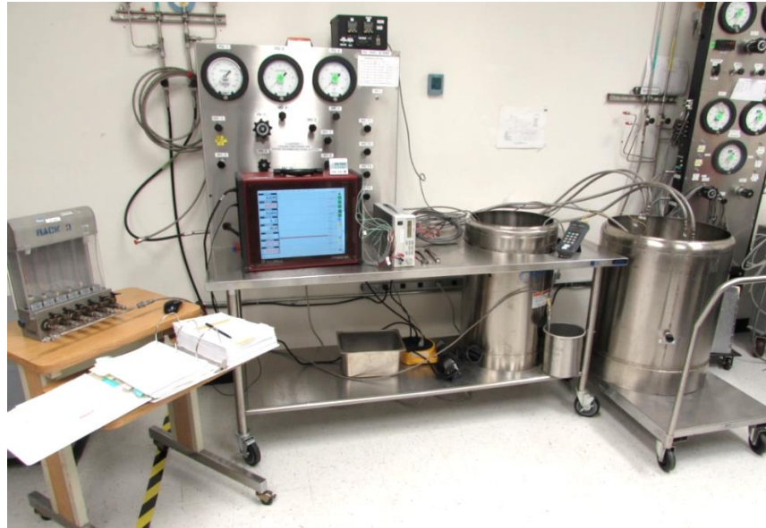
FIGURE 52 AMBIENT LEAKAGE TESTS: TEST SETUP
