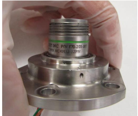
FIGURE 80 SWITCH CONNECTOR (J1)
