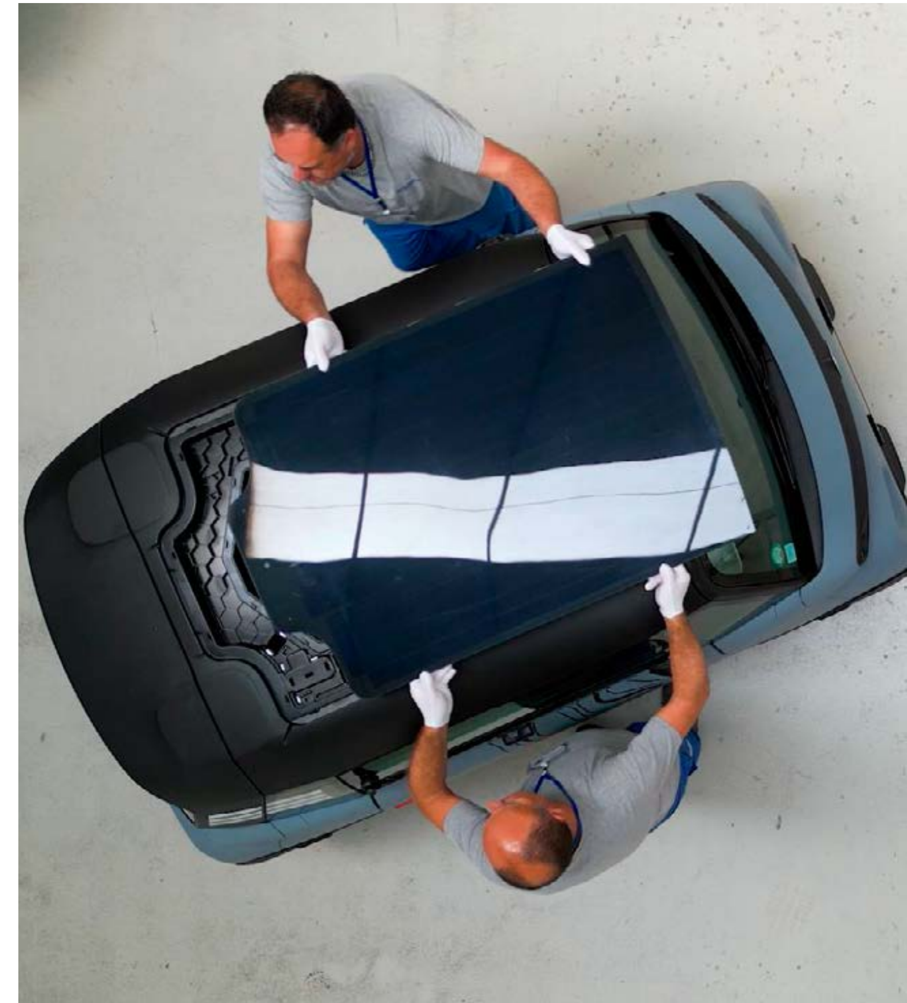
Simoldes Plásticos and Valoe jointly developed a solar roof module made of composites. The picture demonstrates well the lightness of the module, and the installation looks easy too.
