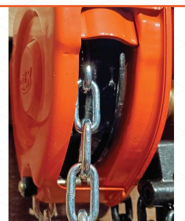
OVERLOAD PROTECTION ADDS AN EXTENDED LAYER OF PROTECTION TO THE USER OF THE HOIST AND THE HOIST ITSELF.
