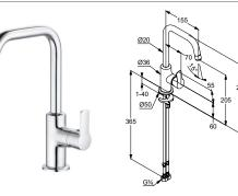
KLUDI PURE&EASY single lever basin mixer DN 15 single hole mounted solid lever ceramic cartridge PCA aerator M 18 x 1 flow rate 5 l/min at 3 bar swivelling spout without pop-up waste flexible hoses G 3/8 rapid installation set spout height lower edge 205 mm chrome 6)
