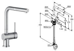
KLUDI L STEEL single lever sink mixer DN 15 swivelling spout, pull-out spout solid lever material: stainless steel single hole mounted flow regulator M 18 x 1 flow rate 8 l/min at 3 bar swivelling spout (110°) ceramic cartridge protected against back flow flexible hoses G 3/8 with shank fastening
