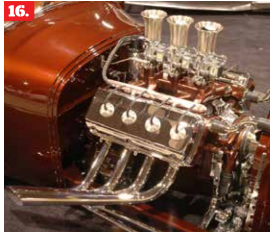
16. Tommy Ivo ran a Vertex with his mechanical Hilborn-injected 322ci stretched to 402ci Nailhead in his iconic T-bucket. Note the clear spark plug wires—not something you would want to run today for street performance and reliability. (Photo by Chuck Vranas)
