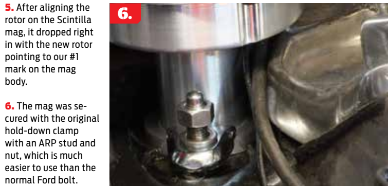
5. After aligning the rotor on the Scintilla mag, it dropped right in with the new rotor pointing to our #1 mark on the mag body.
