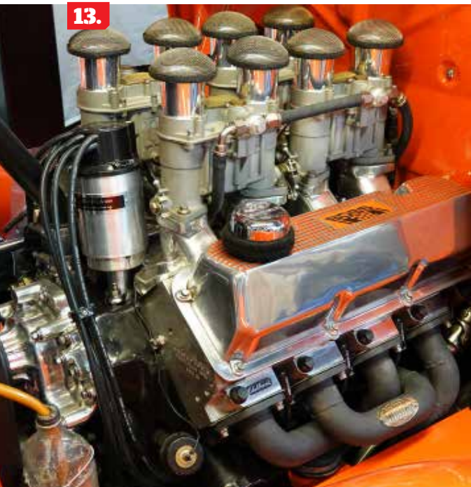
13. With the Eclipse Scintilla-style mag installed and the eight-stack "Weber" throttle bodies, our 351 Cleveland has the perfect '70s vintage vibe yet runs like a new car.
