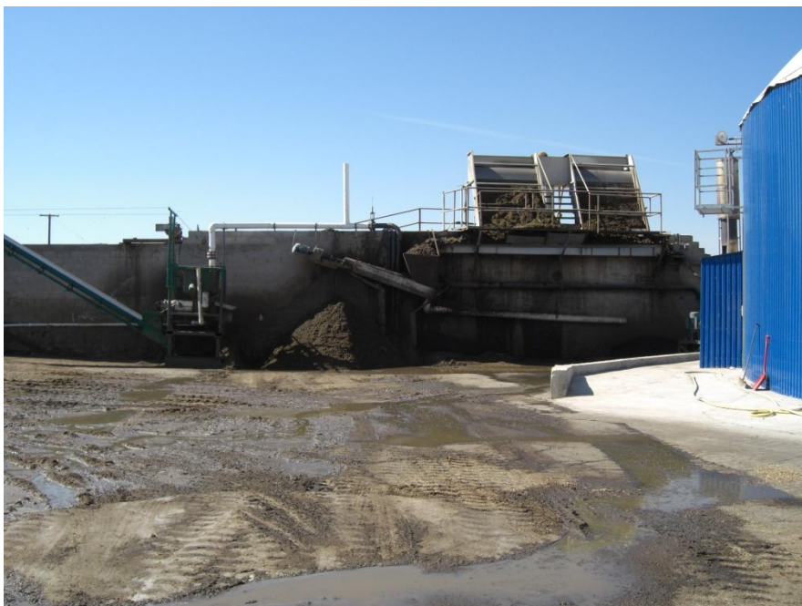
Fig. 8: Separation of digestate into a solid and liquid fraction at Fiscalini Farm (Source: Authors own)
