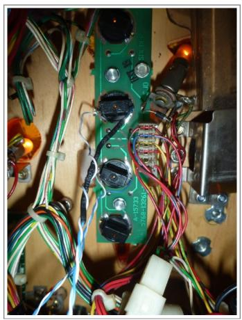
Note: with mods and wiring supplied with the red wire to the positive leg and the resistor to the positive side - the testing phase comes down to a little bit of luck as the games polarity can vary - but at least the LED in the mod is protected with a resistor to the positive leg. A LED typically will only work one way when plugged into the board so is a 50/50 chance that it may work first go, and may need to rotate the socket and then also the LED that plugs into the Matrix socket.
