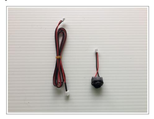
• Cut 2 pieces of 5mm red heat shrink about 30mm long and feed a piece to each end of one cable only and shrink to the cable about 130mm from each end (twist matrix plug end) and about 50mm on the LED end. This will be the Red LED cable.
