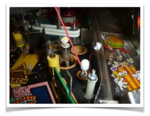
• This step is to ensure the supplied extension lead (3" long) is already connected to the double adaptor lead of the new GI globe. Refer to photo below.
