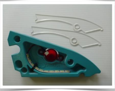
Note: since some people have expressed a desire to experiment with different colour LED's (refer page 17 for purchase links to pick a new / different colour), the pre-installed White LED Strip will be held in place but can be easily swapped over in less than 5 minutes at a cost for \$5 USD for a different colour strip from Comet Pinball.
