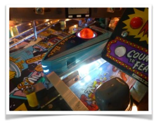
• Lastly re-install the 3 globe light plastic near the snack bar hole to the SS plate with the original nut onto the remaining thread.
