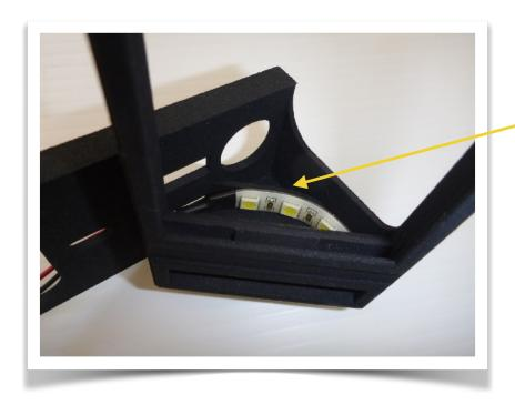
Install the 20 SMD strip around the inside outer edge of the poster retainer as shown below. This
