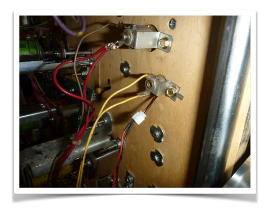
• Then secure the extension lead in a few locations to ensure when lifting / pivoting the playfield the cable does not get caught on anything - note cable ties not trimmed for easier seeing - but make sure to trim back.
