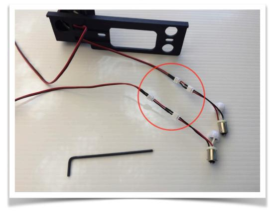
run the game for long periods with the incorrect polarity swap because if it is not working it could damage the LED strips. Allow a max of 10-15 seconds of power time to the game to see if the mod features light up and then turn off if a feature is not working and remove the polarity swap lead as per circled item - but only from the feature lead that is not working.
