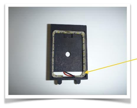
• Fit the 36" extension lead to the poster retainer feed out the back through to poster wide slot.
