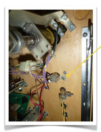
• Then install the Flex SMD into the socket and feed back into the hole but ensure the small extension lead pops out through to the underside of the playfield. Then locate the 36" extension lead and connect up to this new outlet.
