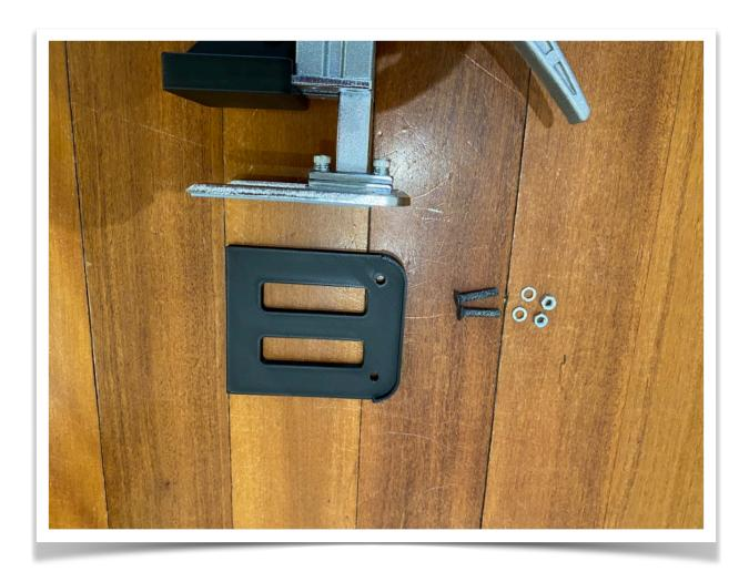
5. Now your Centre Cabinet Jack is ready to use. The thin base is secured to the jack for use at the front of the cabinet and the larger booster base is for use at the back of the cabinet. Simply drop the jack and it's thin base into the booster base and slide into position.
