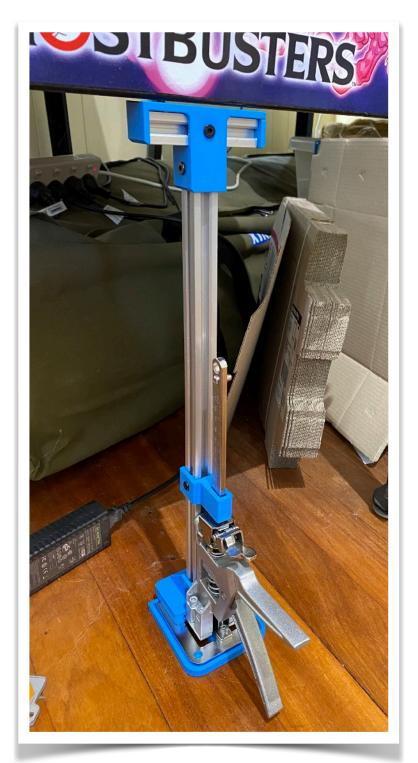
Now line up the Centre Jack Cabinet Support to the bottom of the cabinet. Notice it has an ever so small step at the front and back so the cabinet can not slip off the jack cabinet support once jacked up. And then hand jack so the Centre Jack Cabinet Support is just against the the pinball cabinet.
