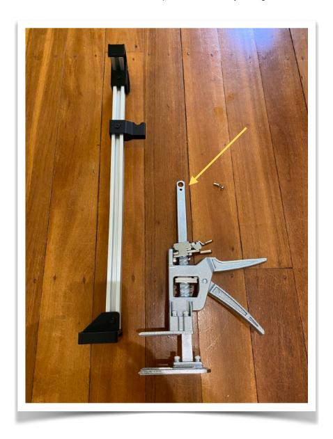
2. Slide the Centre Cabinet Jack Kit onto the jacking lift prong.
