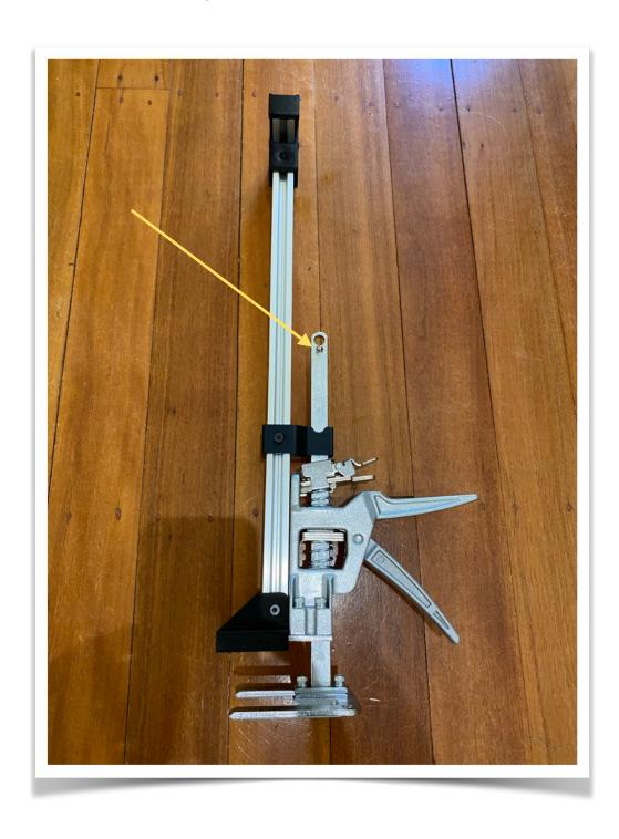
5. You can either double side tape the thin base to the bottom of the jack, bolt on or just slide on. Since this is a recent upgrade a few of the early adopters will need to find some M5 Countersunk x 20mm bolts / washer and nuts or imperial equivalent. These will be supplied to any new kits supplied from April 2024 onwards.
