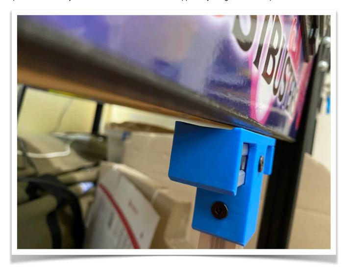
Now you are ready to jack up the cabinet, BUT do not go too high - the higher you go the more the pinball is unstable if pushed or pulled. Once jacked up say 25mm / 1 inch - slide the pin-footie or furniture slider out of the way and adjust your leg leveller up or down and lastly place the pin footie back under the leg leveller and now you are ready to lower your game back to the ground - see next page.
