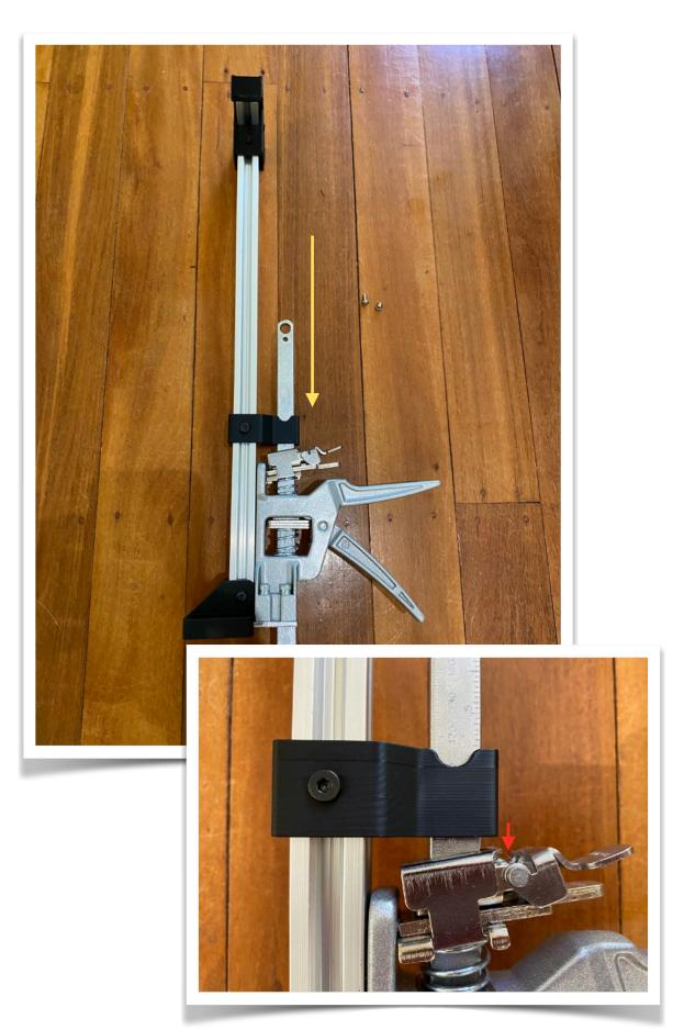
4. Lastly re-install the limit screw at the top of the vertical jacking arm as this limits how high the Centre Jack Lift Arm Slide Guide can go.
