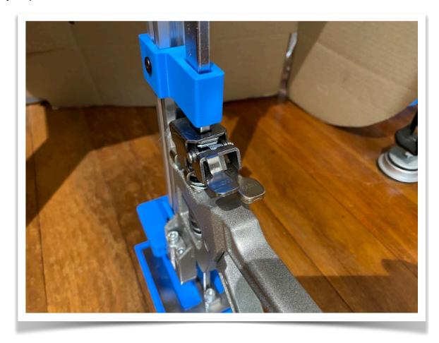
When jacking the back of the cabinet it is a similar process for the back accept cabinets generally are higher at the back of the cabinet so you will need the booster base. Simply place the jack with it's thin base into the recess of the booster base and jack up to the cabinet - ensure to set the jack up vertical and not at an angle and starting to take the load.
