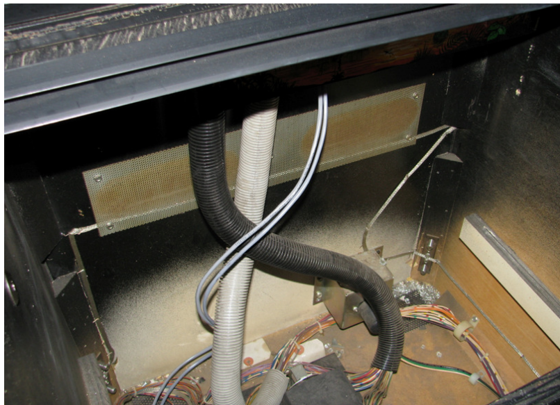
Picture #22 – Slack in Wire Harness
