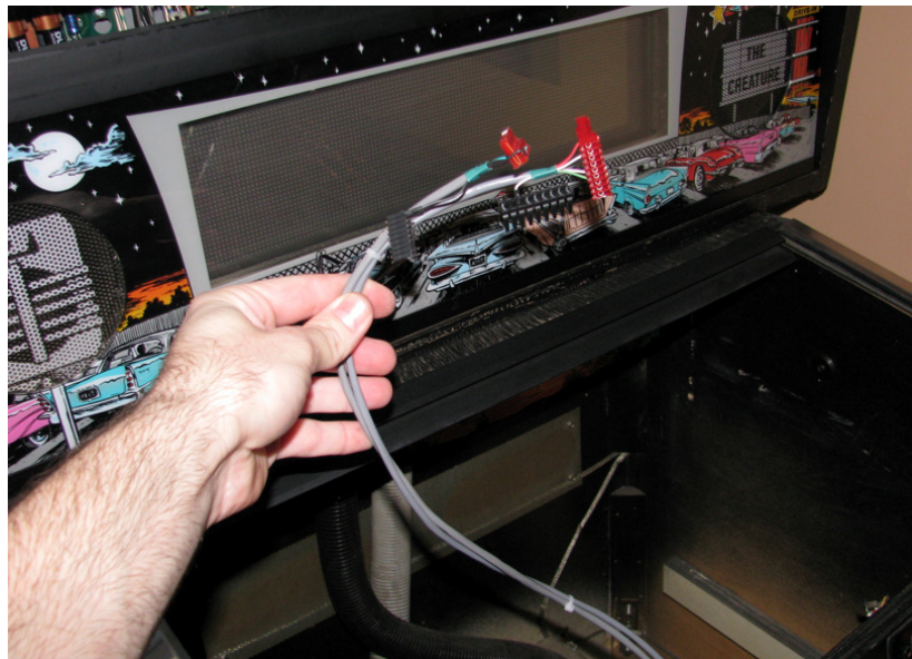
Picture #12 – Portion of MOD Harness that's Routed to Backbox
