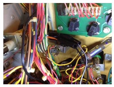
Last, using alligator clips, I connected the drop target flasher" to Input 3 on the PIG 2.
