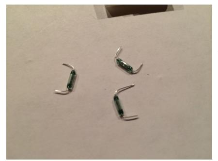
Here is what the reed switches look like with the leads trimmed. I make them nice and short to reduce the chance of them shorting on anything. A reed switch is basically a leaf switch encased in glass that closes when it's in proximity to a magnetic field. Coils are electromagnets.
