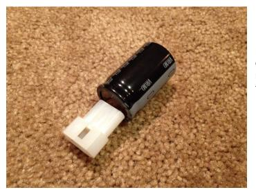
I just soldered .093 pins to a 25v 15,000uf capacitor and snapped them into a plug – making certain to have the negative side of the capacitor connected to the ground pin.
