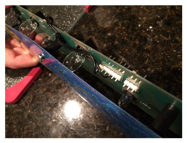
I soldered a connector wire to the back if the 6 pin header, used a sip strap to connect the wire to a post as stress relief, and then ran the wire down to input 2 on the PIG 2.
