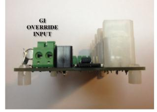
The GI / Override input is a unique input. It has the capability to override the actions of any or all of the outputs.
