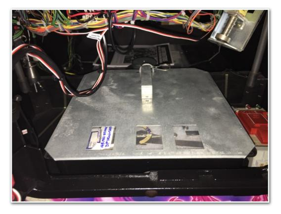
Now take the modded Coin Door Plate with the Coin Box Mount fitted and and slot into the very LHS slot and push it back and it will just rest there has it has a 2.5 degree lean back designed into the bracket and you are good to start enjoying your mod. You can always add a blob of hot glue or a piece of tape to stop the bracket from sliding forward.
