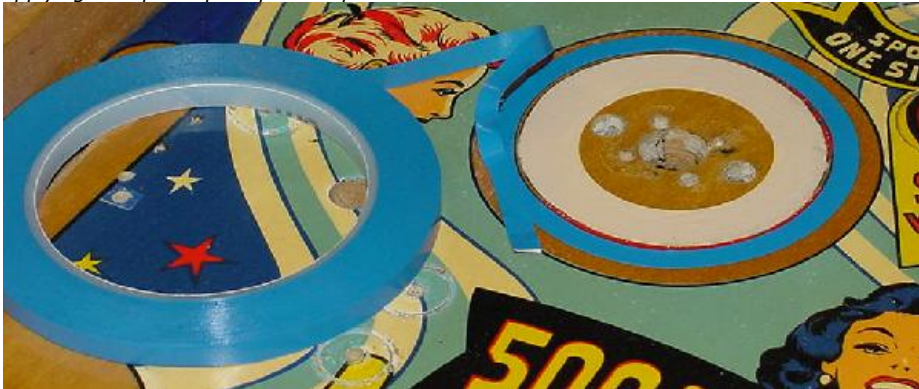
Two layers of blue pinstripe tape are applied, awaiting the new red paint. (This is a 3m product, 1/8" thick 471 plastic pinstrip tape.) Make sure the inner touchup paint has dried a full 24 hours BEFORE applying tape. Otherwise when the tape is removed it can pull-up the fresh white touchup.
