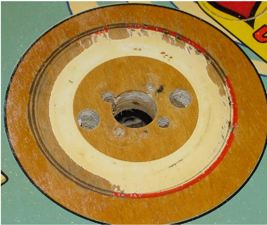
The inner area is painted. Color match is not critical, since the entire area was painted.
