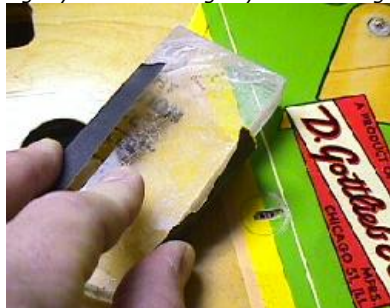
Lightly block sanding dry with 1200 grit.
