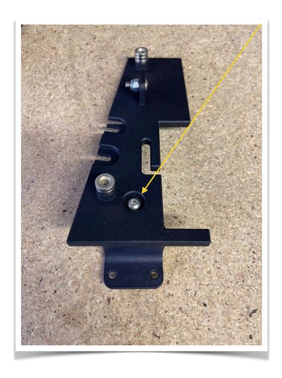
Locate the 2 hex head screws that held the Stern Fire House front mount down as these will be used to install the Fire House Base Bracket to the playfield where the Stern Fire House Front Mount Went and it will look like this once installed.
