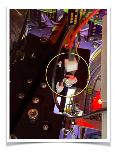
You will notice a very short lead in this power lead - this is the the polarity swap wire. I wire up the accessories with the correct polarity and then stern is correct polarity but the Comet Adaptors are incorrectly wired and this there leds are universal all their leds light up but we need this short lead to make the mod light up.
