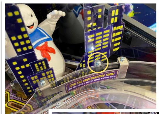
Now you will have enough flex in the ramp to lift and side shift the ramp a little to the right to gain access to the last screw holding the Stern Fire House in place shown with the yellow circle.
