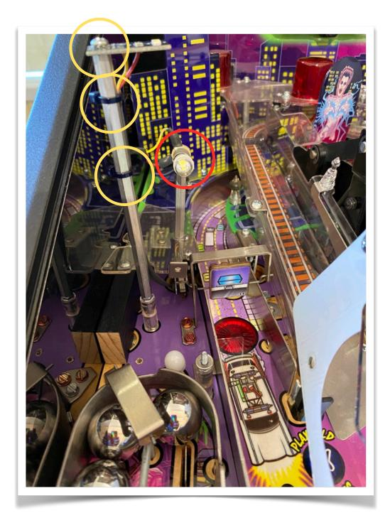
Now twist out the very tall hex post, and the plastic post and also the threaded stud holding down the plastic post.
