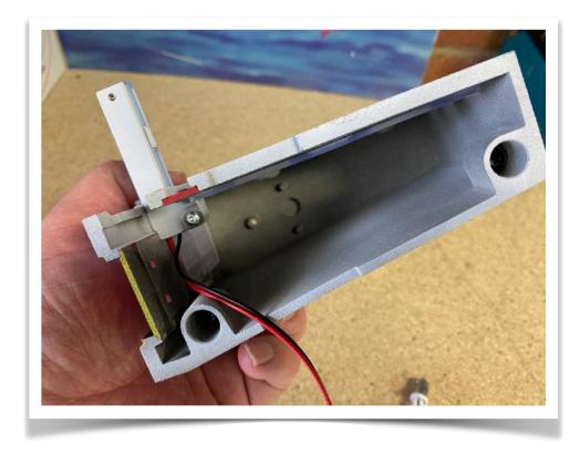
The filter block has a slot in the side to insert the filters so place this side towards the anchoring post / hole like below.
