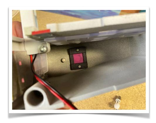
Next place a microfibre cloth on the ramp as you will need to install the stock Stern Flasher board. Insert the supplied bolt through the top of the roof and wiggle any available slack from the flasher board cable and insert into the building and over the bolt. Next place the nut into the Skinny Finger Nut Tool (see below) into the non triangle end and then pass this up into the mod and onto the thread. Then carefully rotate the bolt from the outside and nip up the bolt / nut.
