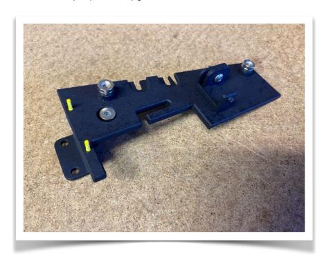
• The Ecto Spinner Topper is slightly different in that I opted to have the main mount made in Black Nylon with no painting required.
