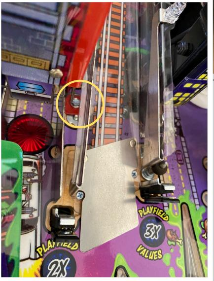
Next you need to remove this 3rd hex head screw that is a little under the ramp (plastic on a Pro). This is probably the most awkward to get to and will require some screws to be removed that hold the ramp in place - see next page.
