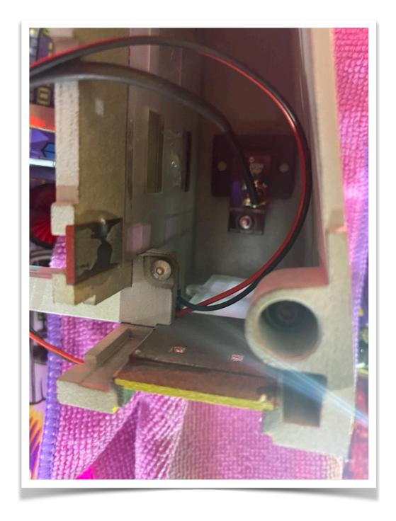
Once the topper is installed re-install the Ecto Light Bar Lens and re-engage the grub screw so it is just flush with the bottom of the bar mount.
