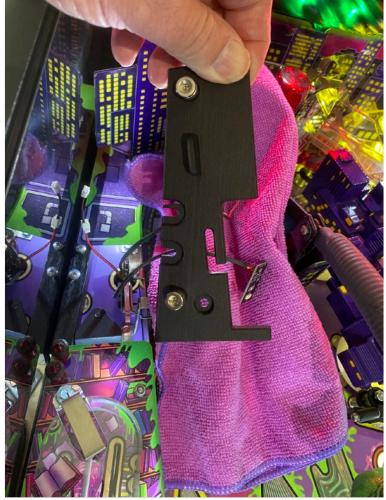
Now locate the base plate. The hole at the front mounts to the bracket you just installed and the 2 slots locate under the 2 screws that are in the side rail. The Base Plate does come with the supplied bolt already mounted to the vertical lug - remove this before mounting one of the original lights.
