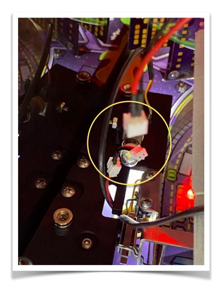
You will notice a very short lead in this power lead - this is the the polarity swap wire. I wire up the accessories with the correct polarity and then stern has correct polarity components but the Comet Adaptors (socket) are incorrectly wired as their leds are universal so not a issue for them as all their leds light up but we need this short lead to make the mod light up as it switches the polarity from the incorrect socket.
