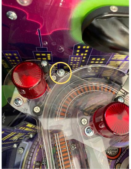
Remove this bolt, washer and spacer from the long hex post and set aside on the cloth.
