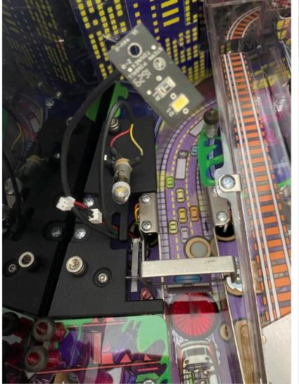
Now lower the base plate so under the screw heads on the side rail. While lowering into place ensure the 3 cables feed into the provided slot - this keeps the cables away from switches and getting pinched when locking the plate down.
