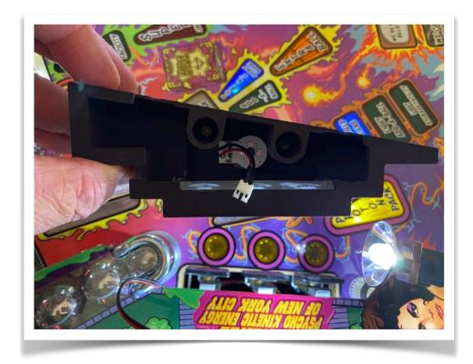
Once installed it will look like this. The Pro (below) is located more central in relation to the targets where as the Premium / LE the library location is governed by the upgraded base plate that needs to cover the large clear space of the graphic plastic so will place a little higher up like the original library but a fraction smaller which I believe is needed as the original was a little over sized.
