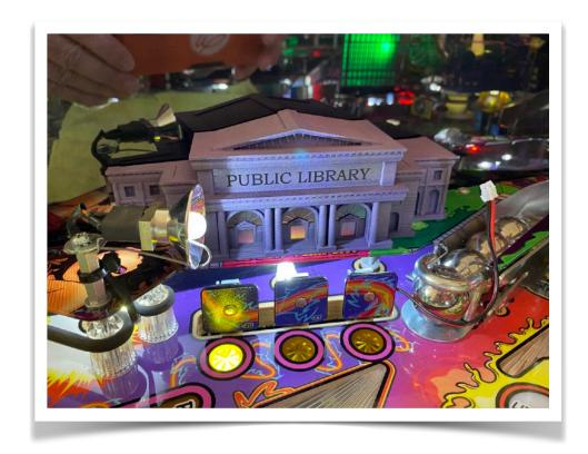
Then connect the extension lead to the Comet star post led lead inside the library.
